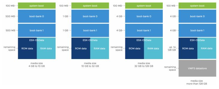
For storage media such as USB or SD devices, the ESX-OSData partition is created on a high-endurance storage device such as an HDD or SSD. When a secondary high-endurance storage device is not available, VMFS-L Locker partition is created on USB or SD devices, but this partition is used only to store ROM-data. RAM-data is stored on a RAM disk.
