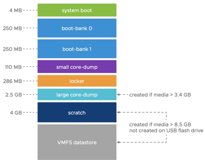
The partition sizes in vSphere 6.x are fixed, with an exception for the scratch partition and the optional VMFS datastore. These are created depending on the used boot media and its capacity.
