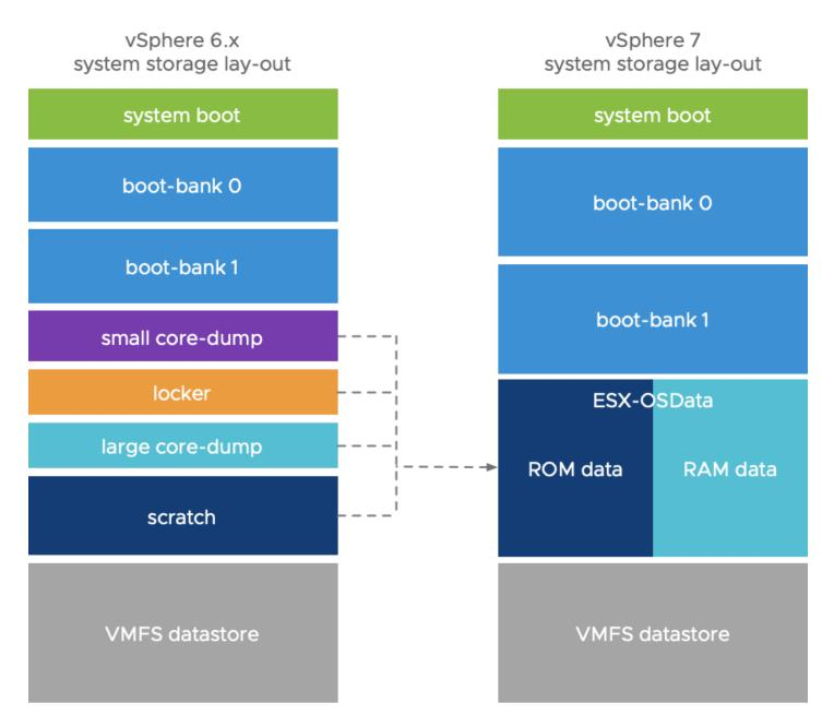
The ESXi 7 System Storage lay-out only consists of four partitions.
