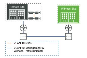
To enable this functionality, the witness traffic is separated completely from the vSAN data traffic. The vSAN data traffic can flow between the two nodes on the direct connect, while the witness traffic can be routed to the witness site over the management network.
