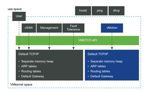
When you configure the traffic services on separate TCP/IP stacks, deploy each traffic service type onto its own network segment. The network segments are accessed through a physical network adapter with VLAN segmentation. Map each segment to different VMkernel network interfaces with the respective traffic services enabled.
