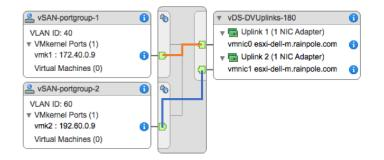
Typically, each uplink must be connected to fully redundant physical infrastructure.
