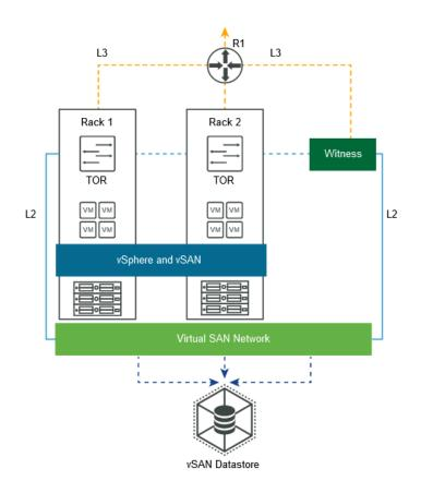
This topology supports deployments with two racks to achieve rack awareness (fault domains) with a vSAN stretched cluster. This solution uses a witness host that is external to the cluster.
