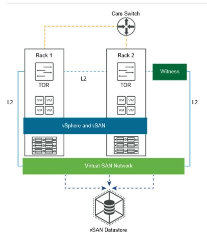
In this example, if rack 1 fails, rack 2 and the witness host provide VM availability. This configuration is a pre-vSAN 6.6 environment, and needs multicast configured on the network. The witness host must be on the vSAN network. Witness traffic is unicast. In vSAN 6.6 and later, all traffic is unicast.
