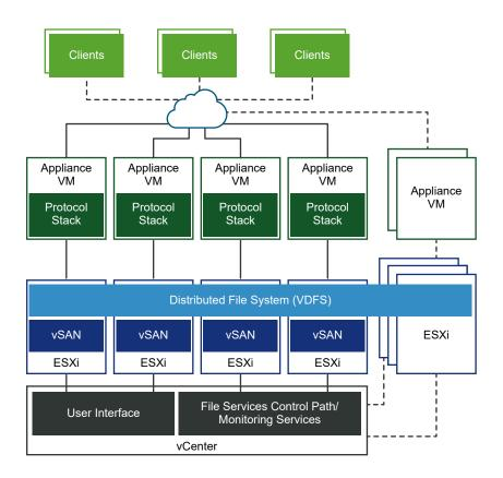
When you configure vSAN file service, vSAN creates a single VDFS distributed file system for the cluster which will be used internally for management purposes. A file service VM (FSVM) is placed on each host. The FSVMs manage file shares in the vSAN datastore. Each FSVM contains an NFS file server.
